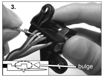
3. Insert each terminal pin into the correct slot with the "bulge" end facing the outer rim of the connector (see 2.a/2.b diagram for connector outer rim definition.)
